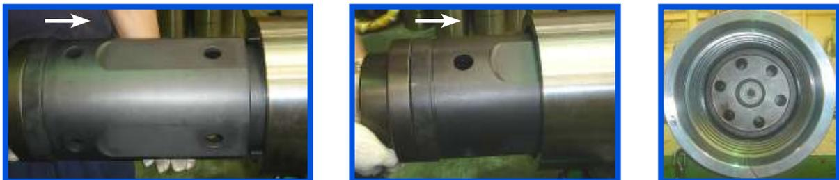
10. First put **Make-Up ring** (Part No. 6) and into Wear Sleeve (Part No. 1) tightly.
