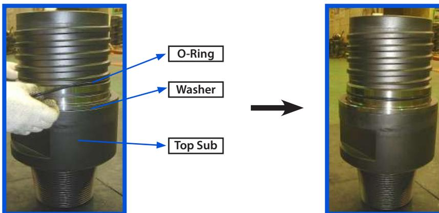
14. Screw the **Top Sub** (Part No.2) with above **Washer & O-ring** into top end of **Wear Sleeve** (Part No.1) tightly.
