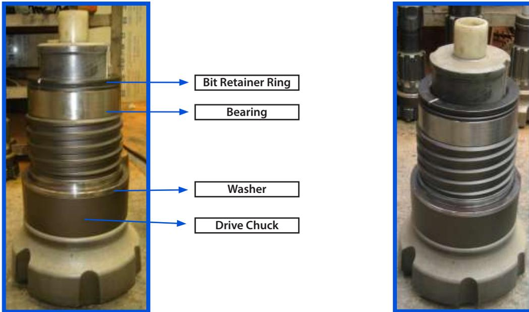
7. Screw the assembled **Drive Chuck** with **Bit** into the **Wear Sleeve** (Part No.1)
