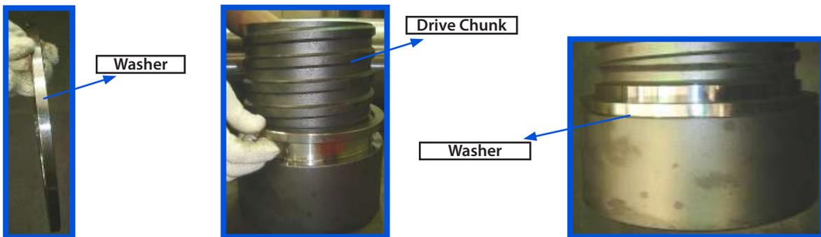
5. Screw the **Chuck** (Part No. 22) into the **Case** (Part No. 1) Matching screw line tightly.
