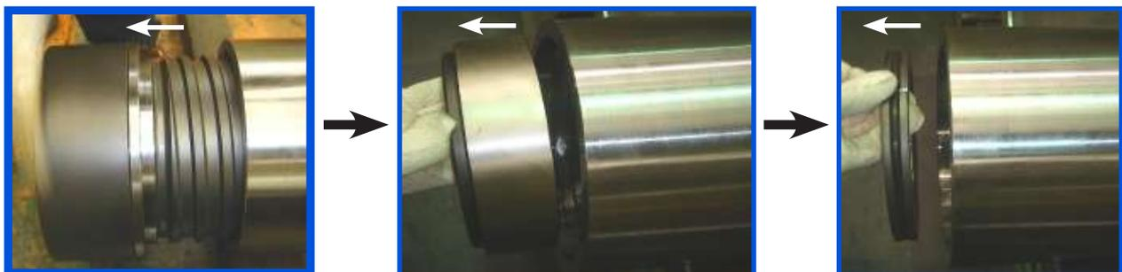
4. Fit down the **Drive Chuck** (Part No. 22) with Washer around Bit as shown
