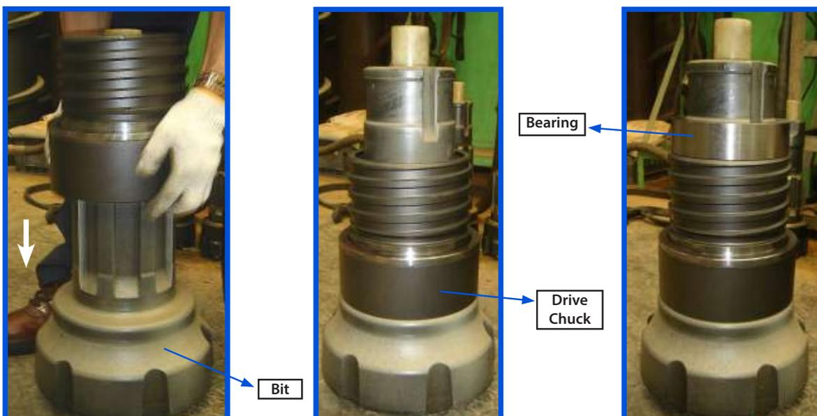
6. Put the **Bit Retainer Ring** (Part No.18) with **O-ring** around **Bit** as shown.
