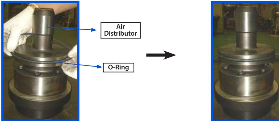
8. And then insert the **Air Distributor** (Part No. 10) with the **O-ring** above into the **Cylinder** (Part No. 12).
